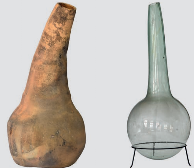
Distilling flasks made of clay and glass found in the attic of the Alte Stadtapotheke
